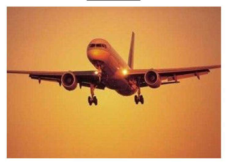
The First Boeing 757 flight was in 1982 and the 757 entered service in January the following year. Subsequent versions to evolve are the 757-200PF Package Freighter, a pure freighter, and the 757-200M Combi. The standard passenger aircraft is the 757-200. The newer version is the 757-300. The 757 has a passenger capacity of 200 to 289, a cruising speed of 530 mph and a range of approximately 3900 nautical miles.
