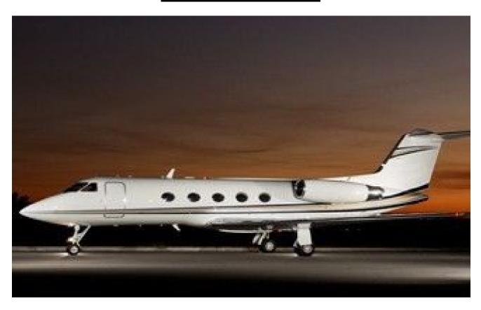
The Gulfstream III is an updated model of the Gulfstream II. It was developed in the late 1970's and first delivered in the early 1980's. Its increased the wing span and surface area allowed for larger fuel tanks, increasing its range. The G-III also has added winglets to reduce drag. It is piloted by a 2 man crew and seats up to 16 passengers. The Gulfstream III cruises at speeds up to 500 knots and has a range of 4,100 nautical miles.
