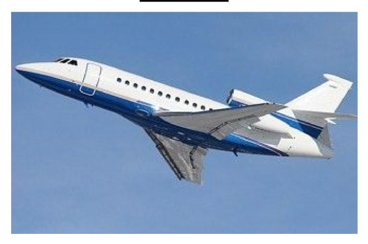
The Falcon 900 is a technologically advanced business jet and first began in 1986. It has has a low/swept wing and 3 rear fuselage mounted engines. The fuselage has 12 cabin windows on each side. The tail has the recognizable number two engine at its base, swept tailfin and mid-mounted swept tailplane. It holds a crew of two and up to 13 passengers. The Falcon 900 cruises at 540 mph and has a range of 4,000 nautical miles.
